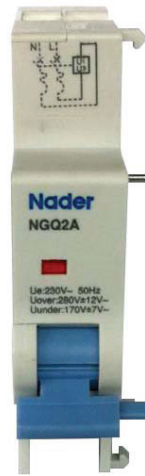
Overvoltage and under-voltage tripper NGQ2A
