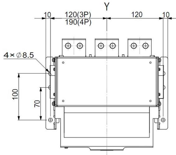
Note: 3-pole breakers X and Y are front cover symmetry axes;
