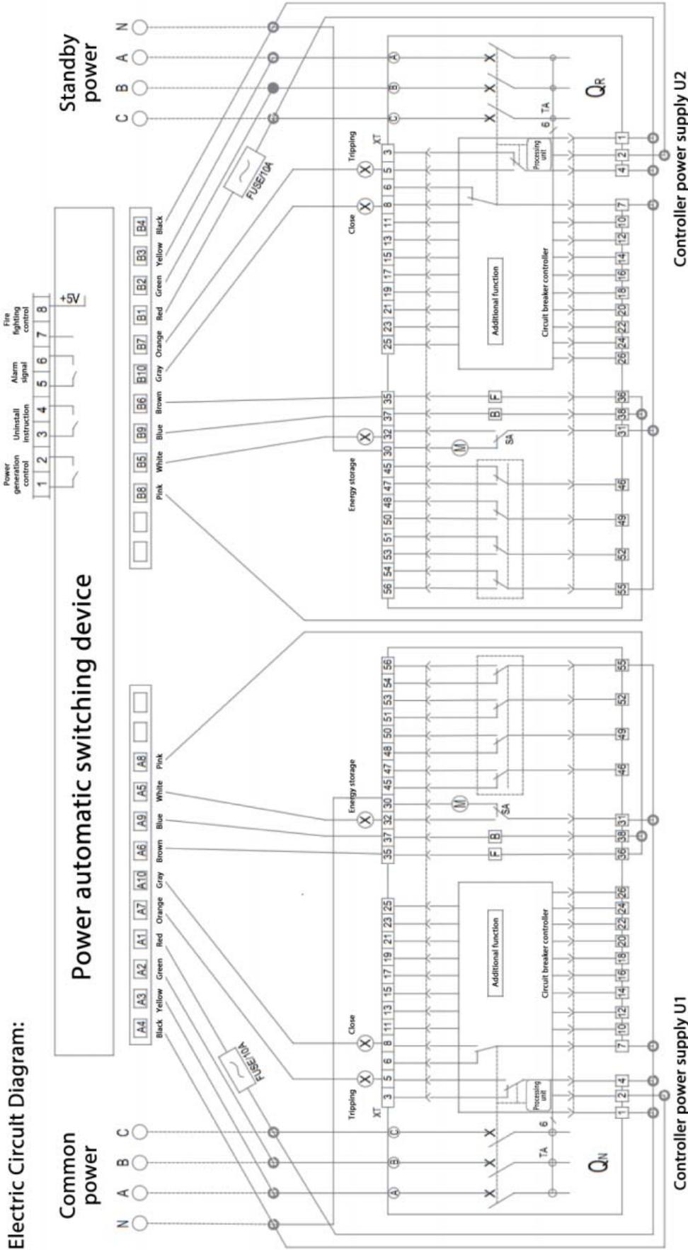
QN - Frequently-used power supply universal low-voltage circuit breaker
