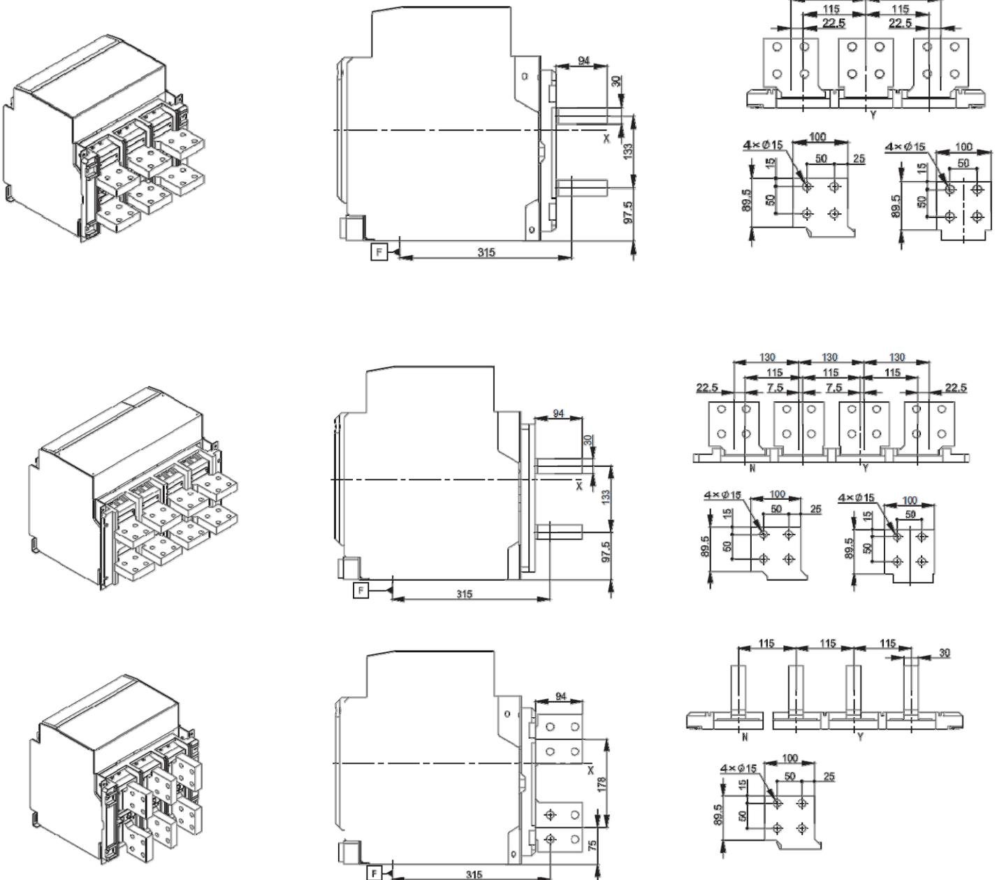
Note: For the 3-pole circuit breaker, X and Y are the symmetric axes of the front cover;
