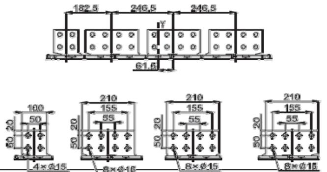
Note: For the 3-pole circuit breaker, X and Y are the symmetric axes of the front cover;
