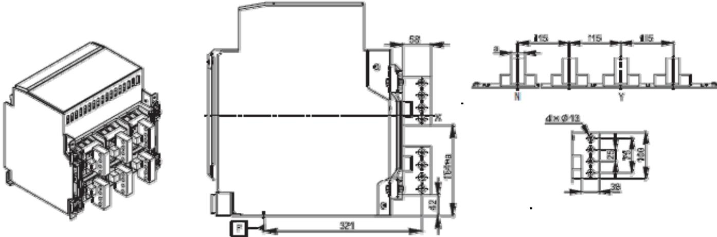
Note: For the 3-pole circuit breaker, X and Y are the symmetric axes of the front cover;
